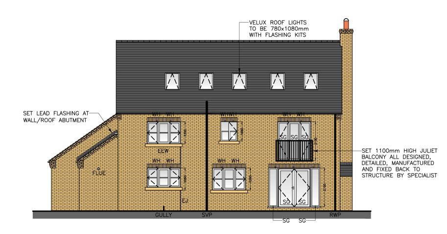
PROPOSED REAR ELEVATION (1:100)EJ = EXPANSION JOINT
